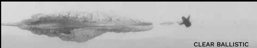
$V_0$ : 360 m/s / 1181 fps. –  $E_0$ : 454 Joule / 336 ftlbs – Test barrel length: 150 mm
