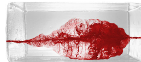
→ Simulated wound cavity in ballistic gelatin: Cal. .30-06 at 200 m
