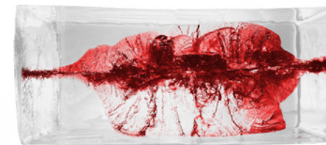
→ Simulated wound cavity in ballistic gelatin: Cal. .30-06 at 100 m
