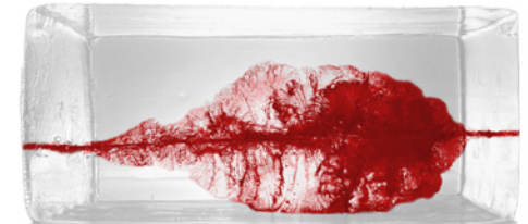
→ Simulated wound cavity in ballistic gelatin: Cal. .30-06 at 200 m
