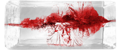
→ Simulated wound cavity in ballistic gelatin: Cal. .30-06 at 100 m
